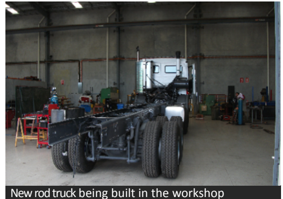
New rod truck being built in the workshop
