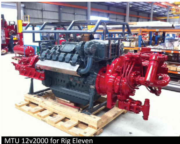
MTU 12v2000 for Rig Eleven
